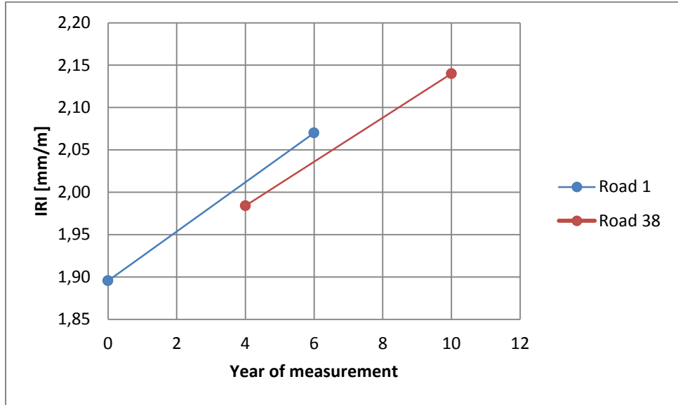
Figure 3-11. Development of average measured IRI for the test sections in Iceland (year 0 corresponds to year of construction).
